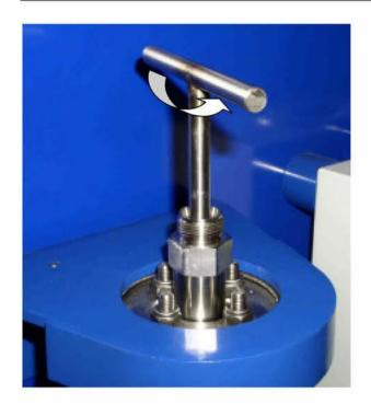
Tighten the sieve insert against the nozzle using the sieve key.
