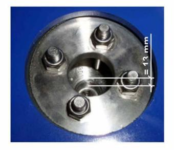
Screw in the sieve insert to such an extent that the screw-in depth into the internal thread is approximately 13 mm.
