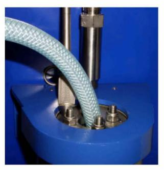
Introduce the suction hose of an industrial suction device into the adsorption container and empty it completely.
