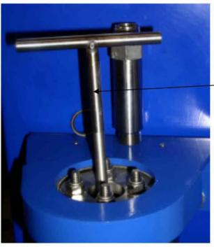
Introduce the sieve key (special tool, not included in the scope of delivery) into the aperture.
