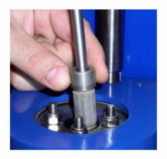
Screw in the sieve insert again using the sieve key.
