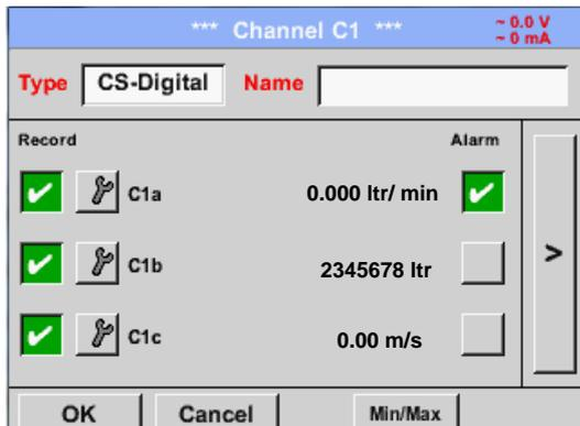
Use the *Record* buttons to select the measurement data that will be stored by **activated data logger**.
