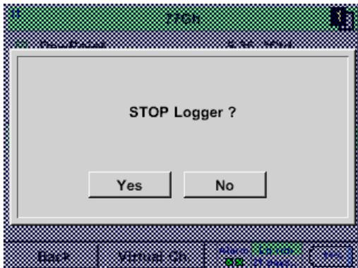
If the data logger is activated, the following window will appear and via pushing **Yes** it can be disabled.
