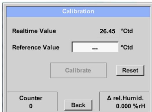
Here, a one-point calibration can be performed.
