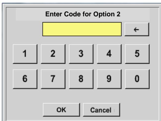
Please enter the Key-Code in the text-field and activate the option by pushing the button *OK*.
