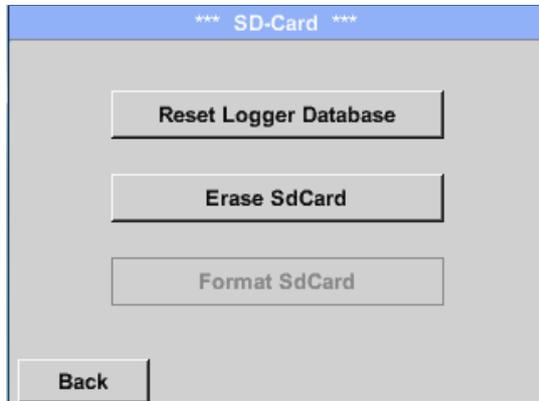
By pressing *Reset Logger Database* all actual stored data on SD-Card will be blocked for use in DS 400. Nevertheless all data are still stored and available for external use only.
