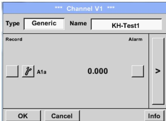
The *Resolution* of the decimal places, the *Short Name* and *Value Name* are found under the **Tool button**
