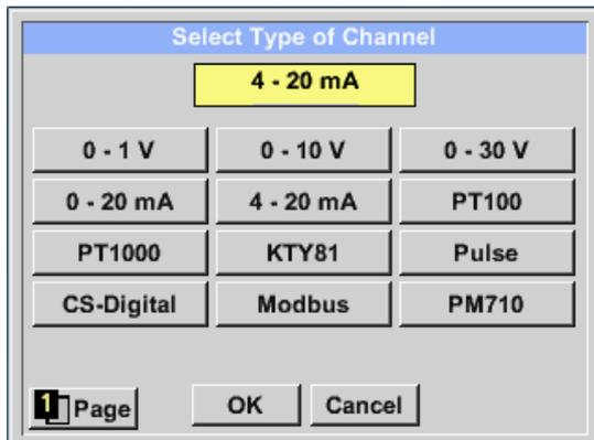
By pushing the button of the required sensor button e.g. 4 -20mA the sensor is selected. Pushing the button **No Sensor** will reset the selection.
