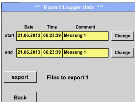
Use the *Change* buttons to adjust a period between *start* and *end*. Stored measurement data in this period are exported.
