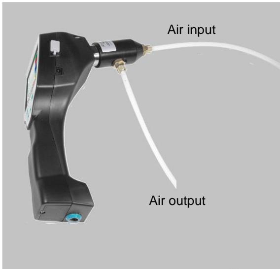
Synthetic granules-dries usually work with a slight positive pressure in the millibar range. Use in this application, with a slight excess pressure, the measuring chamber for synthetic granules dryer (Order No. 0699.3490).
