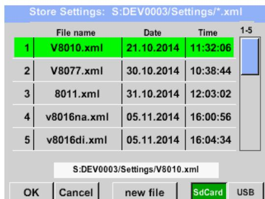
With Export system settings, all existing sensor settings can be exported to a USB stick or to the internal SD card. It stores all sensor settings including recording-, alarm-, graphics-, value- and name definitions. Storing location could be selected using the buttons *SD card* or *USB*.
