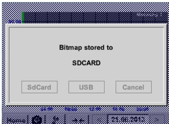
After pressing the Screenshot button a menu (see left) appears where the storage target, USB Stick or internal SD-card, could be selected.
