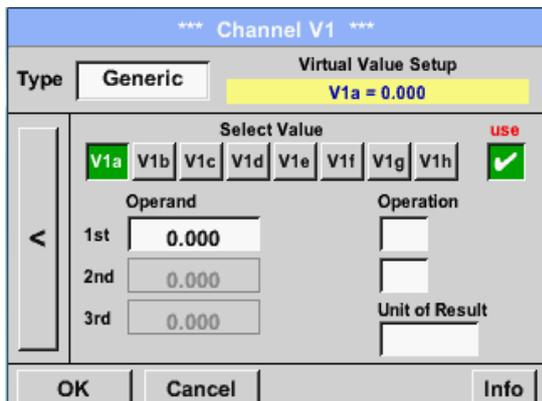
Every virtual value has to be activated by selecting the respective *Value-Button* e.g. *V1a* and pushing of the *Use Button*.
