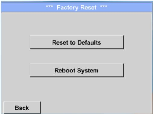
If necessary or required, by pressing the *Reboot System*-button the DP 500/510 DP could be rebooted.
