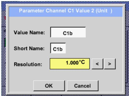
For the recorded *Value* there can be entered a *Name* with 10 characters and later in menu item *Graphics/Real time values* it is easier to identify it. Otherwise the *Name* is, for example, **C1b**. The channel name is **C1** and *a* is the first measurement data at the channel, the Second *b* and the Third *c*. The *Resolution* of the decimal places is simply adjustable by pushing right and left (0 to 5 decimal places).
