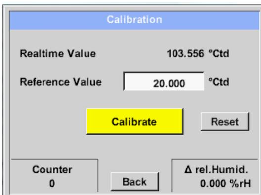
Then by pressing the "Calibration" button taking over the inserted reference value.
