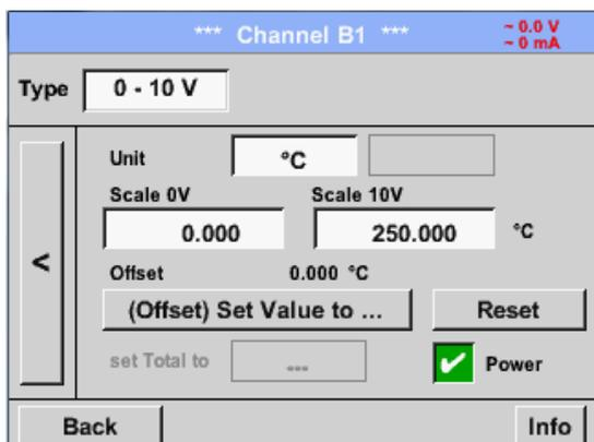
It is possible to define a Offset-Value. With the *Set Value to*-button (*Offset*) you enter it. The positive or negative difference of the *Offset* will be displayed.
