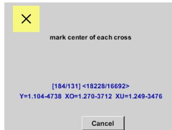
If necessary, the touch-screen calibration can be changed here. Push **Calibrate** and it appears, 1. left above, 2. bottom right, 3. bottom left, 4. right above and 5. in the middle, a calibration cross that must be pushed consecutively. If the calibration finished positive a message "**Calibration successful**" appears and have to be confirmed with **OK**. Is this not the case, so you can repeat the calibration with the help of the **Cancel** and **Calibrate** buttons.
