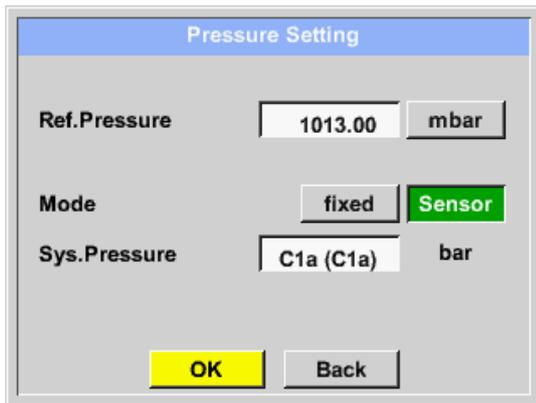
When using an ext. Pressure probe on sensor input C1 (only DP 510) then the **Sensor** button have to be activated.
