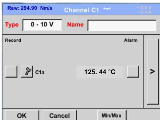
Please see the scale of the sensor (here for example *Type 0 - 10V* corresponds to 0 - 250 °C) from the data sheet of the connected sensor.
