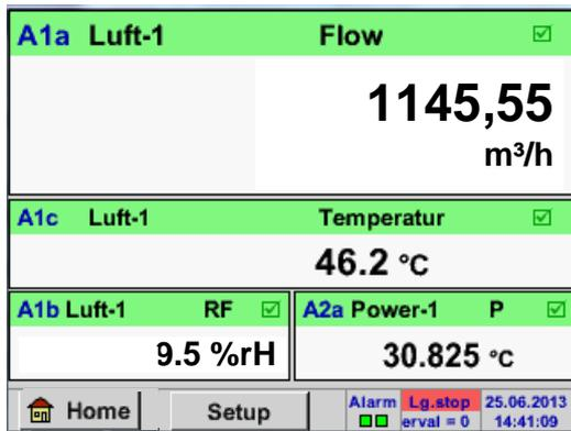
The view *Real time values* allows displaying of 1 to 5 free definable measurement values.
