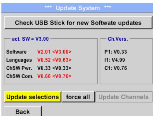
If the DP 500 / DP 510 is correctly connected to USB, and new version available it will displayed.
