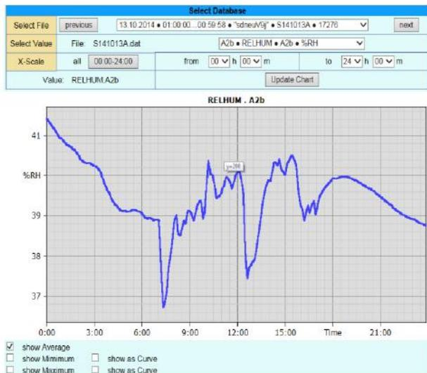
**Select File :** In this drop down field a measurement data file could be selected. With buttons *previous* & *next* could be switched between the files
