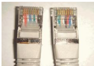
Crossover cable with RJ45-plug
