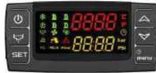
From unit OFF (stand-by) press and release button
