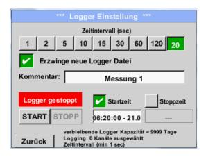
By pressing the Start time button and subsequently pressing the date/time text field below, the date and the start time of the data logger recording can be set.
