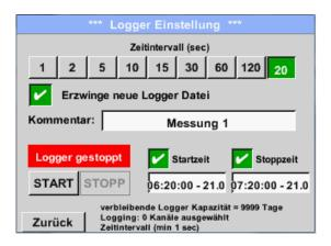
By pressing the *Stop time* button and subsequently pressing the date/time text field below, the date and the time for the end of the data logger recording can be set.
